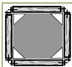
Mainly used in steel shutters by wedging lip between shutter panel and angle iron for automatic attaching. Can automatically be removed from shutters when dismantling and re-used.
