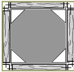
Mainly used for steel shutters by wedging lip between shutter panel and angle iron for automatic attaching. "Plasti-Corner" can automatically be removed from shutters when dismantling and re-used.
