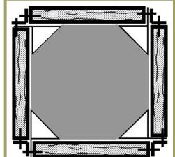
Lip of "Plasti-corner" is slotted as per steel shuttering to take clip and wedge for automatic attaching. When dismantling form work, "Plasti-Corner" comes off automatically and is ready for next use.
